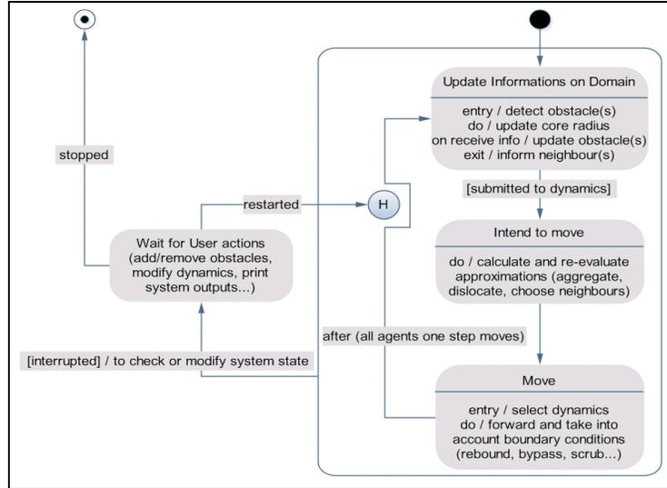
**Figure. 2:** UML State Diagram of an agent-particle in a dynamic system
