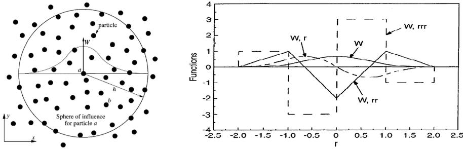
**Figure. 1:** The SPH influence zone of a particle  $a$ , and the distributions of the cubic B-spline function  $W$  and its first three derivatives ( $W, r$ ,  $W, rr$  and  $W, rrr$ ).
