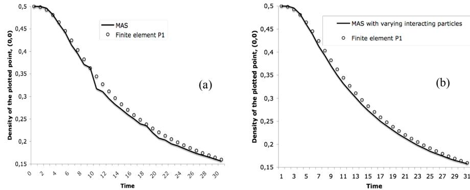
**Figure. 3:** Comparison between the multi-agent model and finite element method on diffusion
