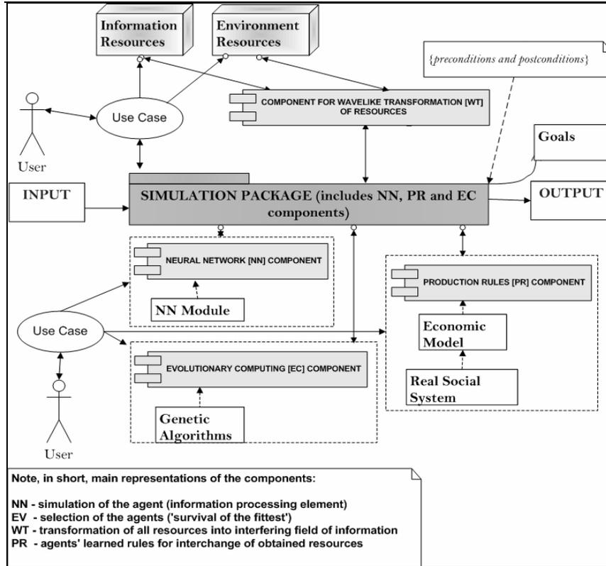
Figure 1. Model setup: UML deployment scheme
