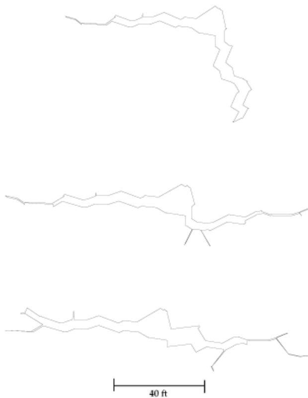
**Figure 6.** Three different fractures for tectonical stresses of 5000 psi along the y axis and 5000 (above), 10000 (center) and 15000 psi (below) for the stress along the x axis which is always the maximum stress.
