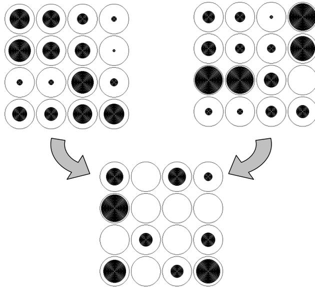
**Figure 1:** The two initial network states shown at top converged to the same stable state shown at bottom. The 16 nodes of the network can each take values from 0 to 1. The values of the nodes are indicated by the radii of the filled circles.
